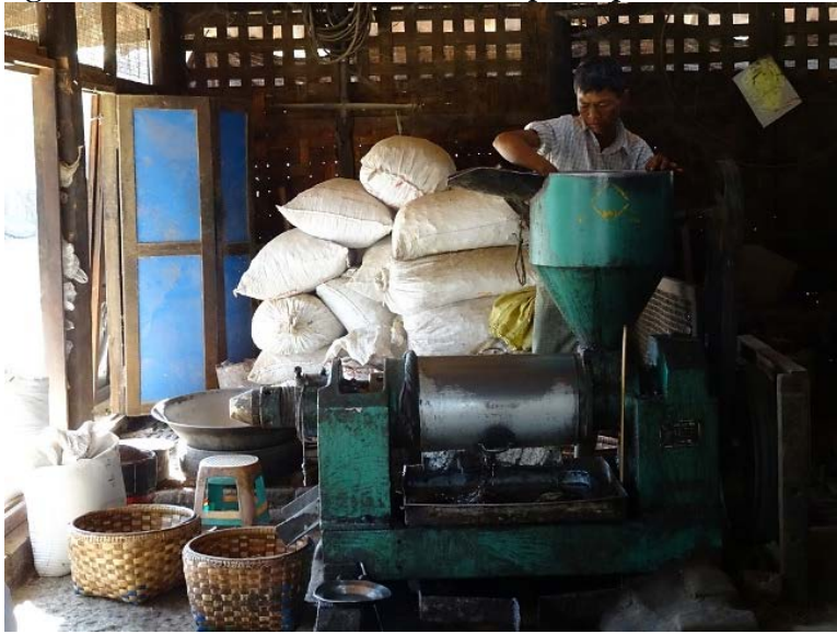
Figure 2c. Large urban mill with expeller press
