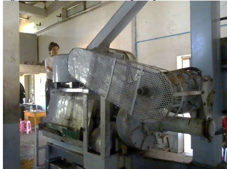
Figure 2d. Large urban mill with expeller press and automatic feeder
