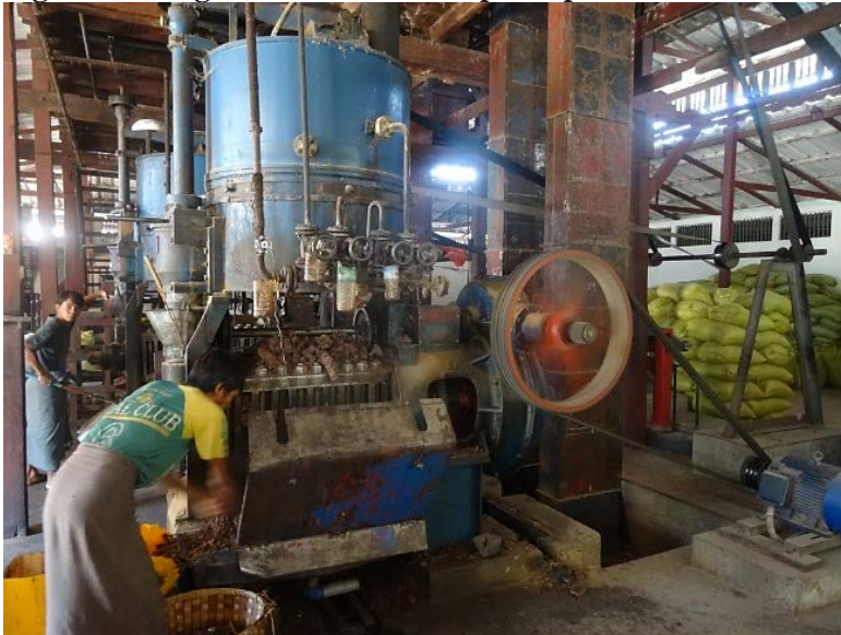
Figure 2c. Large urban mill with expeller press
